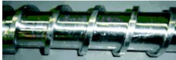
Fig 1. Long pitch conveying screw that facilitates low shear in an extruder.
