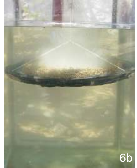
Fig 6. Feed spilling out during various steps (a-e) in the immersion and retrieval of the tray
