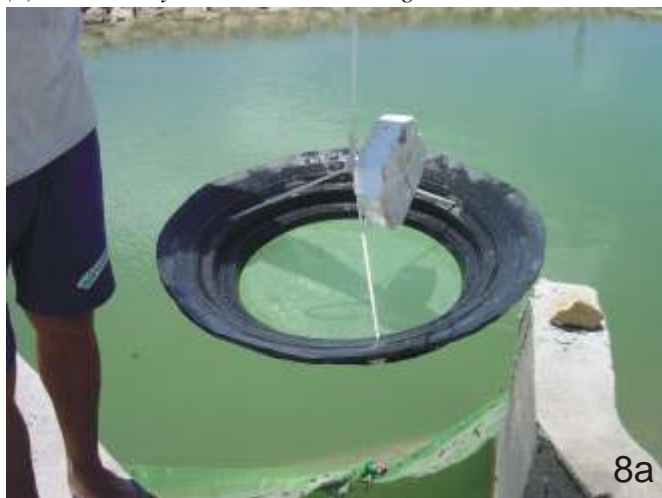
Fig 8. Improvements in tray design to minimize spill out: (a) deeper trays; (b) tray has a PVC feet for smoother landing; and (c) double buoys to slow down sinking rate.
