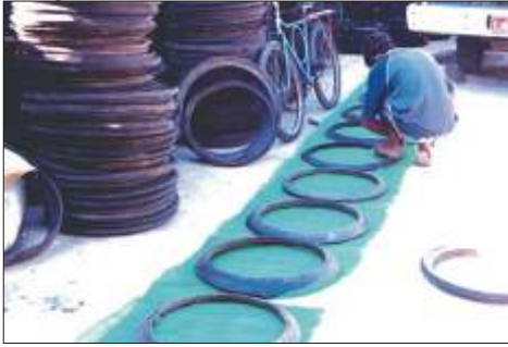
Fig 5. Crafting of trays in Northeast Brazil using old tires.
