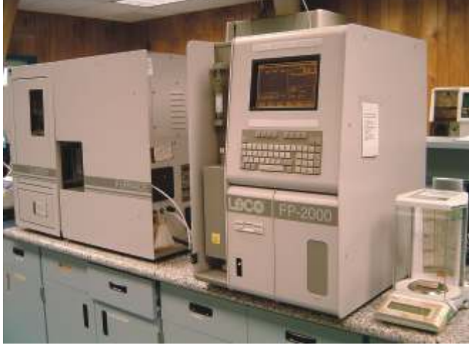
LECO FP 2000 Protein analyzer analyses nitrogen by the Dumas combustion method. The sample is combusted at 600 C and all gases except nitrogen is removed by a series of scrubbers. The nitrogen is then equilibrated with Helium at NTP and measured as percent nitrogen. Automation enables doing 40 samples at the rate of 5 - 6 minutes/sample.
