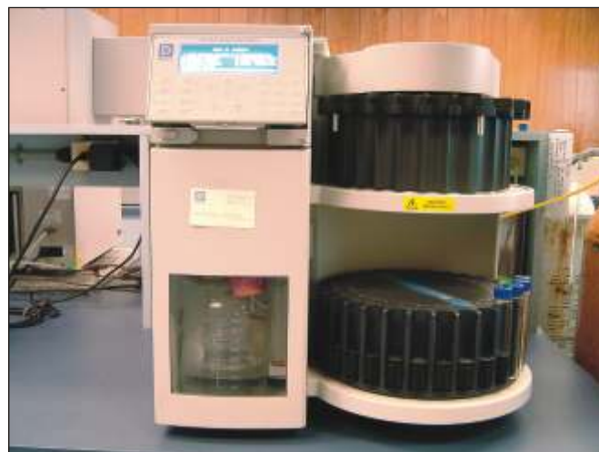
Dionex Accelerated Solvent Extractor is used for determination of crude fat. Petroleum ether (10 mL is used as a solvent and the extraction takes place in a hermetically sealed metal container at 105 C at 140 psi. One sample is completed in less than 10 minutes and this model does 21 samples automatically.
